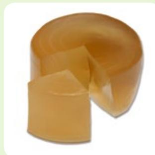
Gel BP85 1:12 heated at 80 °C for one hour
