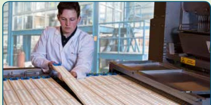
*Gummies are deposited in flexible silicon molds. The absence of starch makes the process completely clean.*
